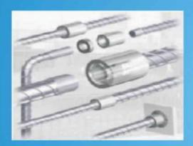
Upset parallel threaded couplers are suited to projects which require high volumes of couplers. They produce a full strength joint in the rebar connection. The ends of the bars to be joined are cut square and enlarged by cold forging to increase their core diameter and so ensure that the joint is stronger than the bar. The couplers are usually supplied attached to the reinforcing bar.
